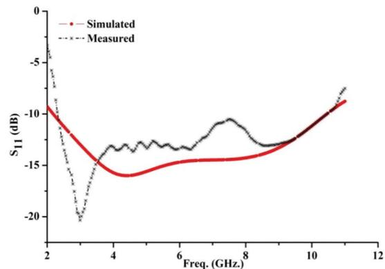
**Fig. 4.** Reflection coefficient of the final optimized MPA
