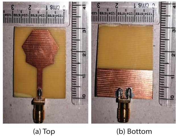
Fig. 2. Dimensions of the fabricated MPA, (a) Patch view and, (b) Ground view
