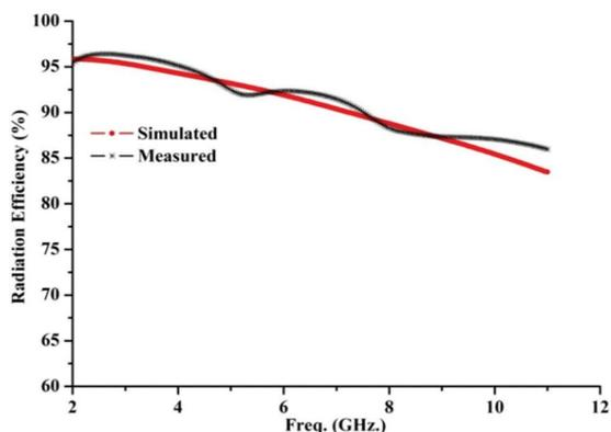
**Fig. 5.** Radiation efficiency of the final optimized MPA
