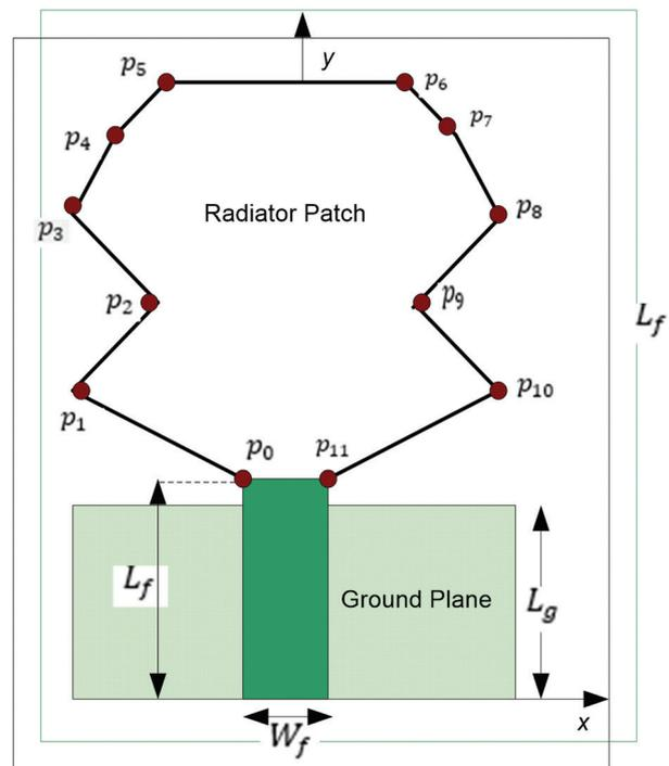
Fig. 1. Initial target irregular-shaped MPA design.
