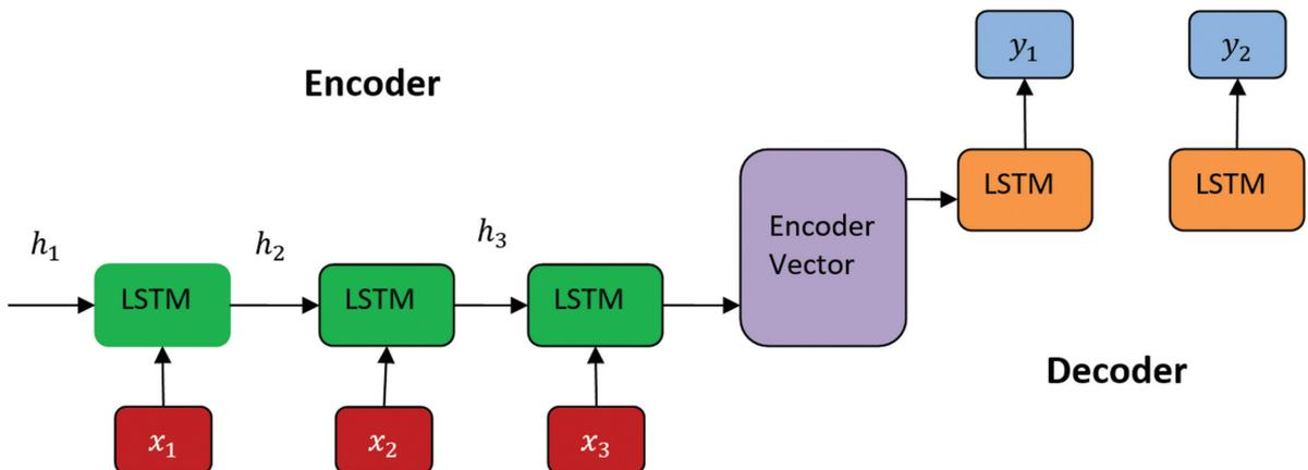
Fig. 3. LSTM based encoder and decoder network
