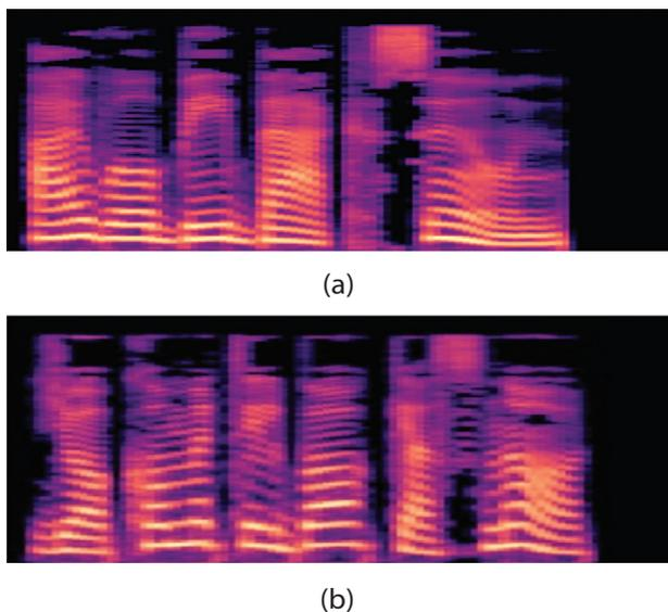
**Fig. 5.** Mel Spectrograms (a) for English sentence "I am suffering from fever" and (b) equivalent in Swedish
