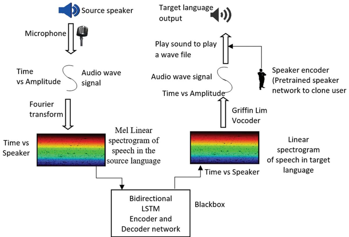
Fig. 2. Functional flow of STS conversion module
