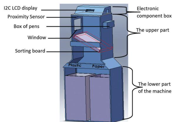
Fig. 2. Machine's design
