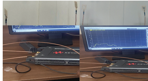
Fig. 12. Free space measurement set up
