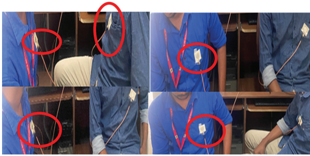
Fig. 16. Measurement set up for off body communication (different bodies)
