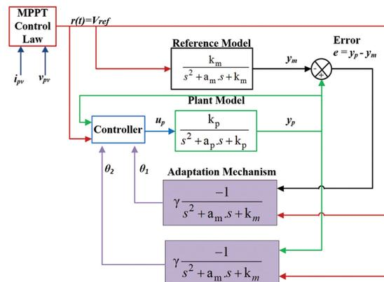
Fig. 6. Proposed MRAC controller architecture
