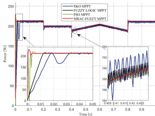
Fig. 13. Simulation results of four MPPT controllers with variable temperature and constant irradiation (1st profile)
