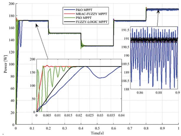
**Fig. 11.** Simulation results of four MPPT controllers with variable irradiation and constant temperature
