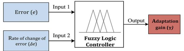
Fig. 7. Fuzzy control input and output variables
