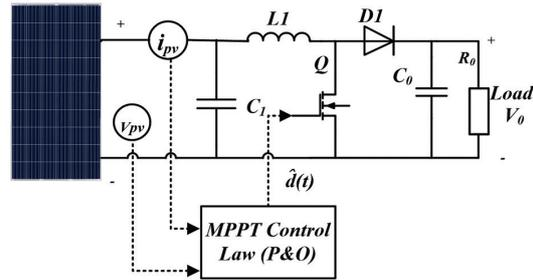
**Fig. 2.** Photovoltaic system schematic diagram
