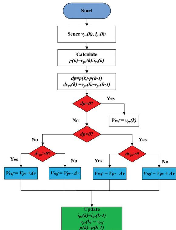
Fig. 5. Voltage Setpoint calculation
