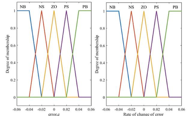
Fig. 8. Membership functions of two inputs
