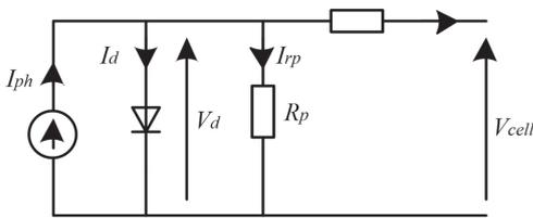
**Fig. 1.** PV circuit equivalent model
