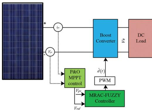
Fig. 4. Photovoltaic system with the suggested MPPT control configuration
