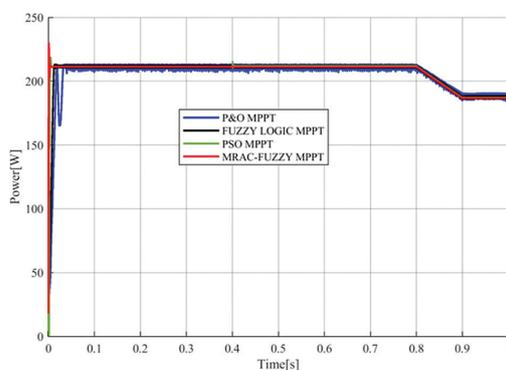
Fig. 14. Simulation results of four MPPT controllers with variable temperature and constant irradiation (2nd profile).
