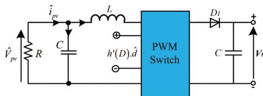
**Fig. 3.** Small-signal model of the photovoltaic output converter circuit
