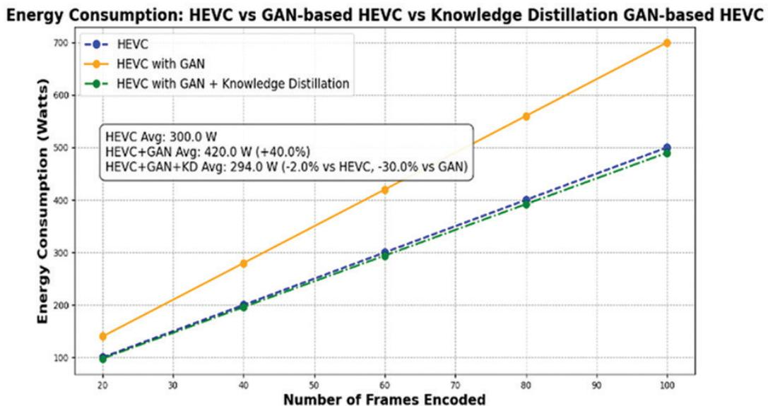
Fig. 3. Energy Consumption between HEVC, GAN-based HEVC, and Knowledge Distillation GAN-based HEVC
