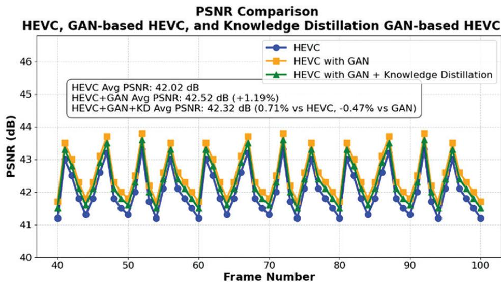
Fig. 4. PSNR values comparison between HEVC, GAN-based HEVC, and Knowledge Distillation GAN-based HEVC
