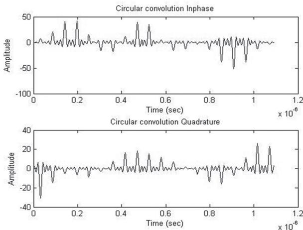
**Fig. 6.** Signal after circular convolution with RRC
