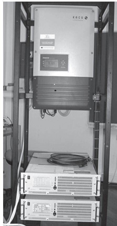
Fig. 1. Laboratory set up of a PV emulator
