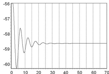
**Fig. 8.** Remaining generator load angle in the case of one generator outage
