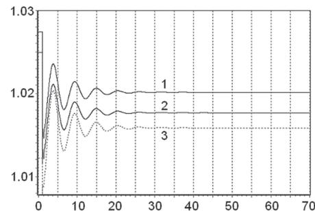
**Fig. 7.** Bus voltages in the case of one generator outage: 1 – voltage on the generator bus, 2 – voltage on the bus of the consumer closest to the generators, 3 – voltage on the bus of the consumer closest to the infinite bus
