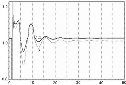
**Fig.10.** Bus voltages in the case of a short circuit at the generator bus: 1 – voltage on the generator bus, 2 – voltage on the bus of the consumer closest to the generators, 3 – voltage on the bus of the consumer closest to the infinite bus
