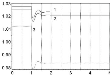
**Fig. 4.** Bus voltages in the case of infinite bus outage: 1 – voltage on the generator bus, 2 – voltage on the bus of the consumer closest to the generators, 3 – voltage on the bus of the consumer closest to the infinite bus
