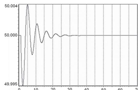
**Fig. 9.** Remaining generator frequency in the case of one generator outage
