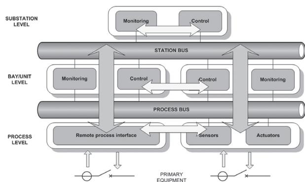
**Fig. 5.** SAS structure with data and information exchange
