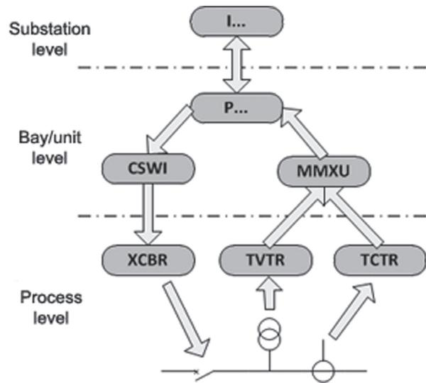
**Fig. 9.** Process information flow between logical nodes
