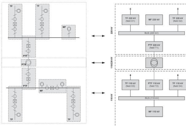
**Fig. 2.** An example of substation decomposition into technological units and technological modules
