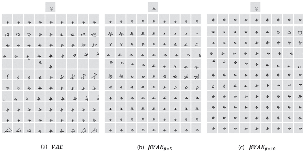
Fig. 8. The first row shows the input image, and the second row shows the corresponding reconstructed images for computing the repeatability of the model. Rows 3-12 show the latent transversal performance of the model. The latent transversal performance of each model, each row shows the code, and columns show the transverse in that particular code with all other codes kept constant. The fifth column in each figure shows the reconstructed instance and their transversals generated based on this.
