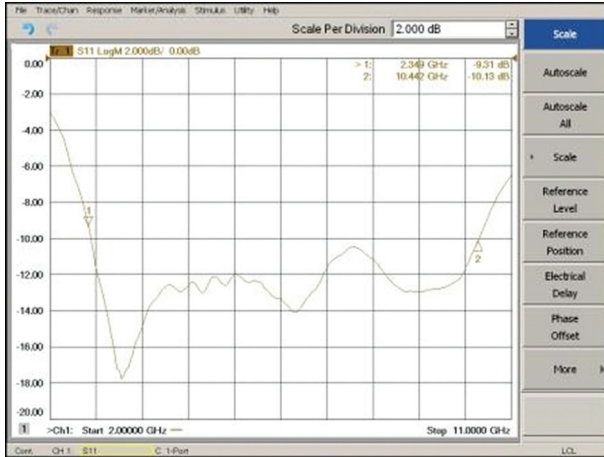
Fig. 6. Reflection coefficient on VNA of the final optimized MPA
