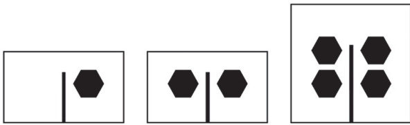
Fig.1. Evolution stages of the proposed single layer proximity fed 2x2 array antenna (a) stage one (b) stage two and (c) stage three
