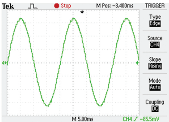
Fig. 8. Output line voltage waveform for 31-level inverter employing SHE technique at m_I = 0.7440 .
