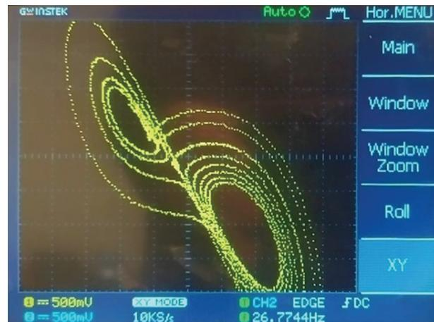
**Fig. 9.** The Lorenz Attractor XY on the oscilloscope
