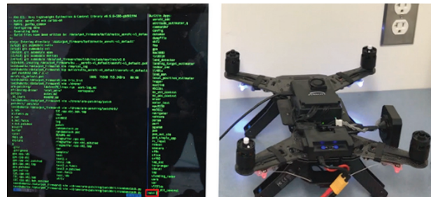
Fig. 11. Result after applying stack memory diversification against PX4-based drone. The screen on the left side indicates internal command/communication operates without problem after patching. Right side of the picture shows LED blinking of the UAV that indicates its normal operation.
