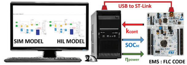
Fig. 6. The proposed HESS 's EMS Hardware-in-the-loop ( HIL ) architecture
