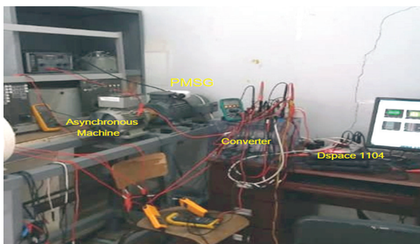
Fig. 4. Wind turbine emulator system in the test bench
