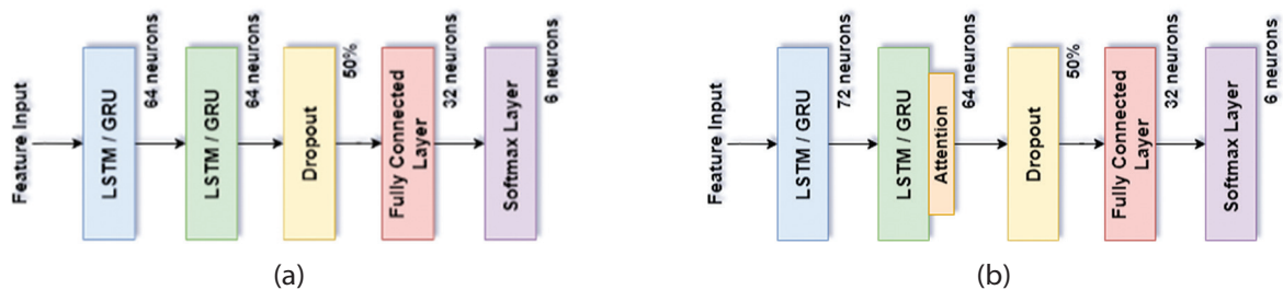
Fig. 4. Two stacked layers model architecture (a) without attention (b) with attention
