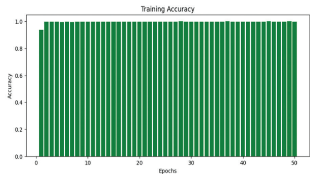
Fig. 8. Training accuracy used EfficientNet model and Adam Optimizer
