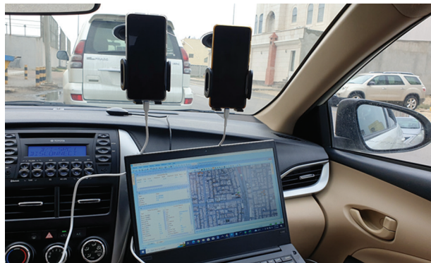
Fig. 7. The TEMS tool setup for field drive test measurements
