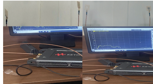
Fig. 12. Free space measurement set up
