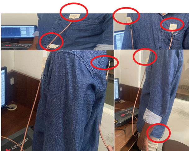
Fig.14. Measurement set up for on body communication (same body)
