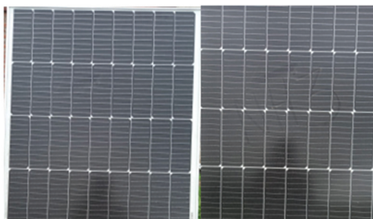
Fig. 5. Panel cleaned (left) and panel without cleaning (right)
